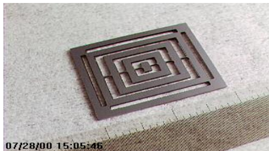
Figure 1. Balanced torsionally vibrating mechanical oscillator.
