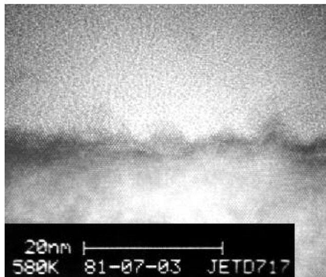
Figure 17. TEM micrograph of the 20x2 nm superlattice after RTA annealing.
