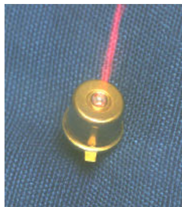
Resonant-cavity LED at 650 nm shining bright and exhibiting a record signal modulation speed of over 300 MHz. Courtesy: ORC / TUT
